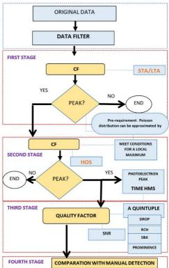
*Flowchart for the four-step algorithm*
