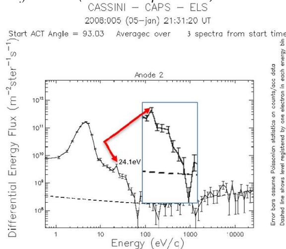
Note: Cassini CAPS-ELS data from the T40 Titan flyby. Six-second averaged (three spectra) differential energy flux (DEF) spectrum starting at 21:31:20: UT. The dashed line indicates the single count level of ELS. The arrow in each spectrum points at the 24,1eV photoelectron peak. Error bars assume Poissonian statistics on counts/acc data.
