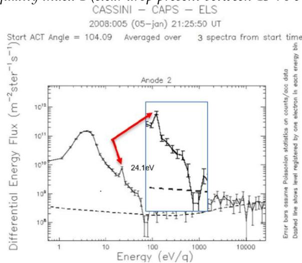
Note: ELS data from the T40 Titan flyby. Six-second averaged (three spectra) differential energy flux (DEF) spectrum starting 21:25:50 UT. The dashed line indicates the single count level of ELS. The arrow in each spectrum points at the 24,1eV photoelectron peak. Error bars assume Poissonian statistics on counts/acc data.
