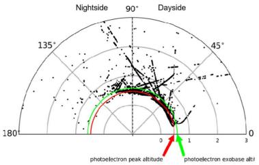
Note: The radial distance from the center shows the distance from Titan in Titan radii (RT = 2.574 km). The angles shown are SZA (Solar Zenith Angle). The photoelectron peak altitude (~1.200 km) and the photoelectron exobase altitude (~1.500 km) are shown as red and green lines, respectively.
