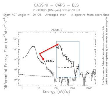
Note: ELS data from the T40 Titan flyby. Six-second averaged (three spectra) differential energy flux (DEF) spectrum starting at 21:32:36: UT. The dashed line indicates the single count level of ELS. The arrow in each spectrum points at the 24,1eV photoelectron peak. Error bars assume Poissonian statistics on counts/acc data.
