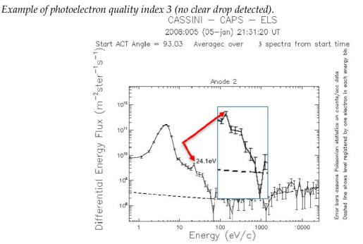
Note: Cassini CAPS-ELS data from the T40 Titan flyby. Six-second averaged (three spectra) differential energy flux (DEF) spectrum starting at 21:31:20: UT. The dashed line indicates the single count level of ELS. The arrow in each spectrum points at the 24,1eV photoelectron peak. Error bars assume Poissonian statistics on counts/acc data. **Source:** Own elaboration
