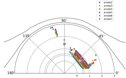
Note: The radial distance from the centre shows the distance from Titan in Titan radii (RT = 2574 km), and the angles show the SZA (Solar Zenith Angle). The position of anode N has been shifted sideways by (N-2)\*0,1 RT to distinguish it clearly from the neighbouring anodes. The grids below 1 RT indicates the photoelectron peak altitude and the photoelectron exobase altitude, respectively. Saturn's nominal magnetospheric plasma flow comes from the top during this flyby.
